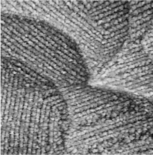
Fig. 4. 500 \times 500 \text{ nm}^2 STM topographic image of 10 ML Co deposited on Au(1 1 1)/mica at RT, as-prepared.
