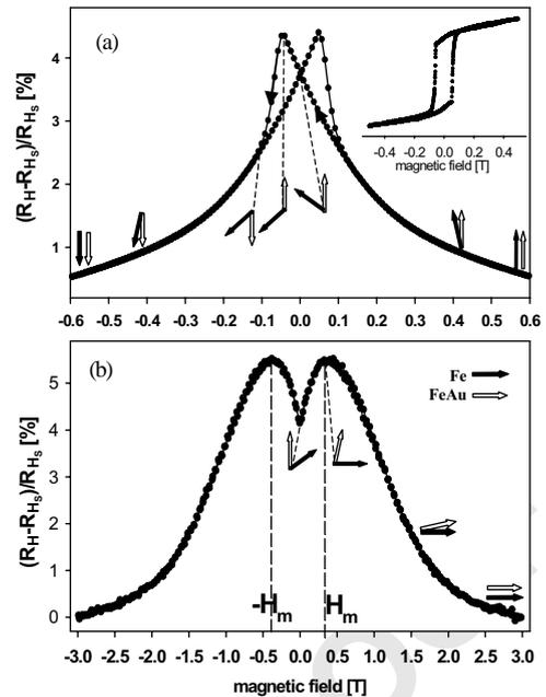
56 Fig. 1. GMR curves measured at 10 K for the  $[\text{Fe}_3/\text{Au}(001)_9/$
