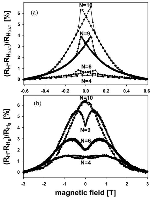
Fig. 2. GMR curves measured as a function of  $N$  for the  $[\text{Fe}_3/\text{Au}(001)_N/(\text{Fe}_1\text{Au}_1)_3/\text{Au}(001)_N] \times 2$  multilayers at 10 K with the magnetic field applied in the normal direction (a) and an in-plane direction (b). The thickness of the Au spacer layer measured in the number  $N$  of Au(001) atomic layers is indicated.
